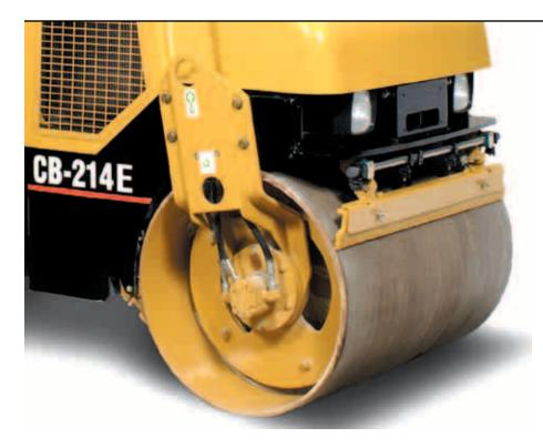
**Drum edges.** Specially designed drum edges help eliminate marks on deep lifts or when turning.
