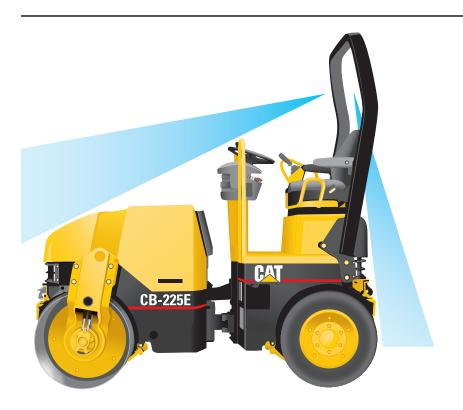
**Forward visibility.** Excellent forward visibility allows the operator to see objects 0.58 m high and 1 m in front of the machine.
